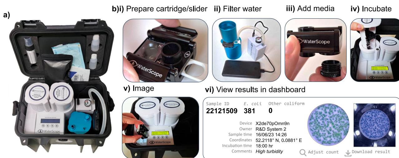
Fig. 1 | Overview of the WaterScope test kit. a Key components shown packed inside the system's case, weighing 6 kg with a size of 29 cm × 23 cm × 26 cm. b Key steps required for a single E. coli test. Note that a single power bank provides
